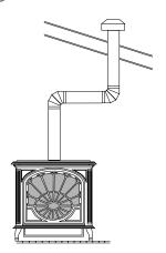
Figure 22 - Vertical Venting Through Ceiling Using Two 90° Elbows
